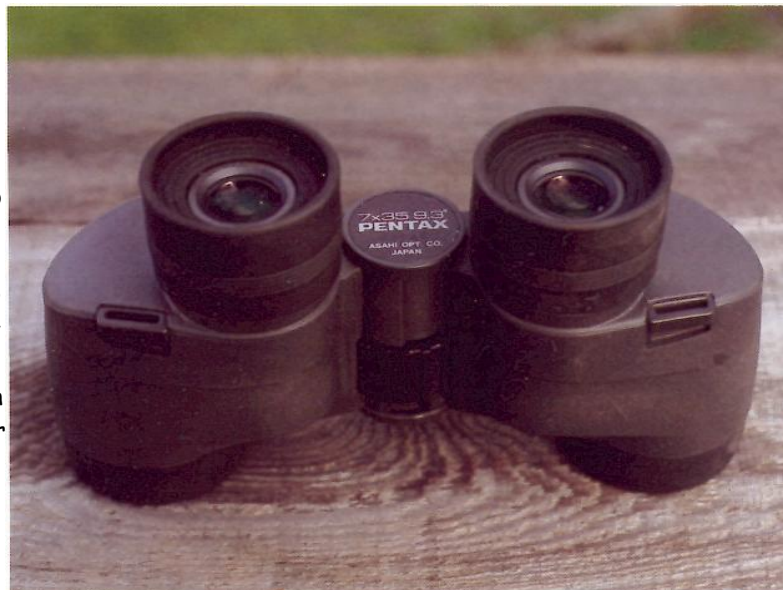
The Pentax 7x35 PCF is a typical general purpose binocular. Visible between the two eyepieces are numbers denoting magnification, size of the objective lens, and width of the field of view.
