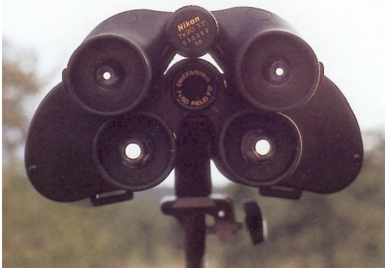
The circles of light visible in the eyepieces of these two binoculars are called the exit pupils. Both binoculars have the same magnification. The Bausch & Lomb 7x50 Discoverer, below, delivers much more light than the compact Nikon 7x20 Travelite M, above, but the Nikon is much smaller and lighter.
